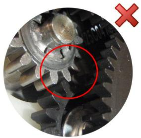
12. Attach the APE cable as shown below. Ensure cable does not foul on any of the APE gears.
