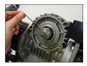
8. Use the provided M4 hex head taptite to drive in and out of the hole shown below, to form a thread. Use a Phillips head style screwdriver.
