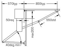
Ensure the angle between the primary and secondary arms is always greater than 40 degrees. The gate hinge should be no more than 200 mm forward of the mounting face of the drive.
