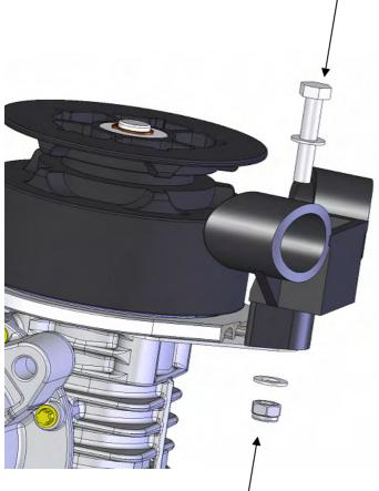
Place the packer and the chain guide over the exposed hole in the dovetail brackets. Insert the Hex head bolt, through a washer, then into the assembly. Fasten underneath with a washer and nylon lock nut.
